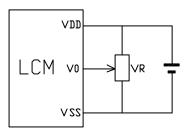
$V_{DD}$ -V<sub>0</sub>: LCD Driving voltage VR: 10k-20k
